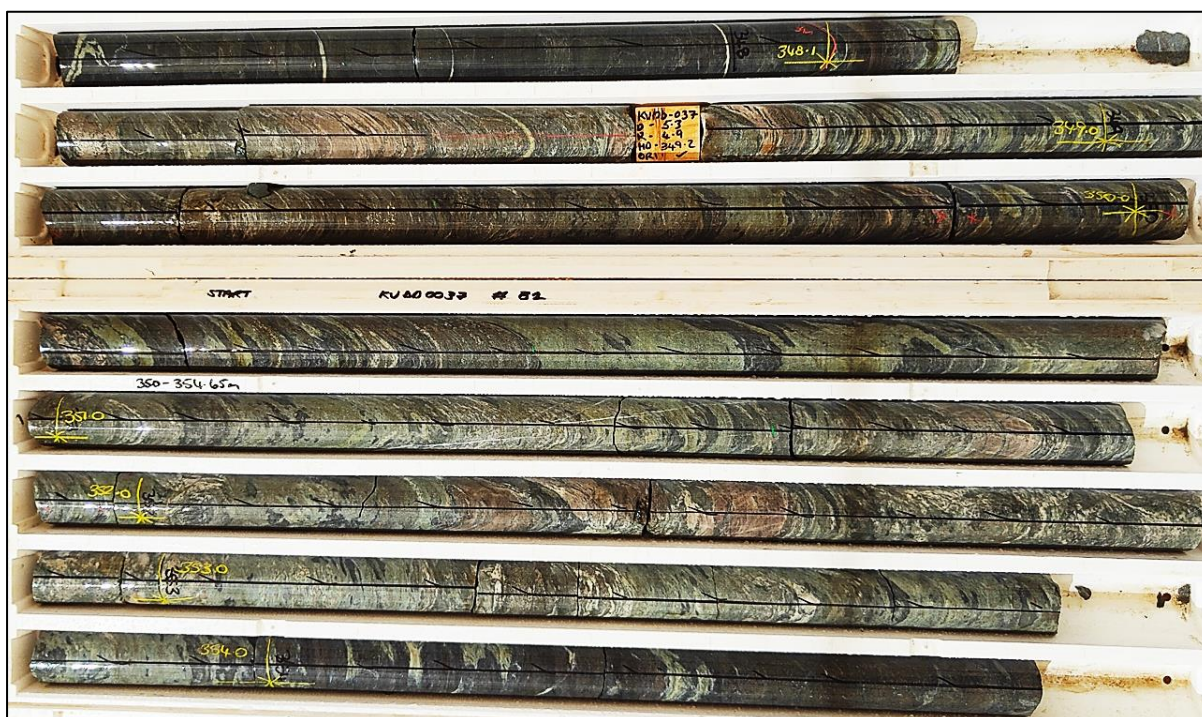
Figure 1: Core from KVDD0037 (347.5-354.6m shown) displaying altered and sulphide bearing rocks typical of the main ductile shear zone which carries the Au-Ag mineralisation at the Coffey Deposit.
