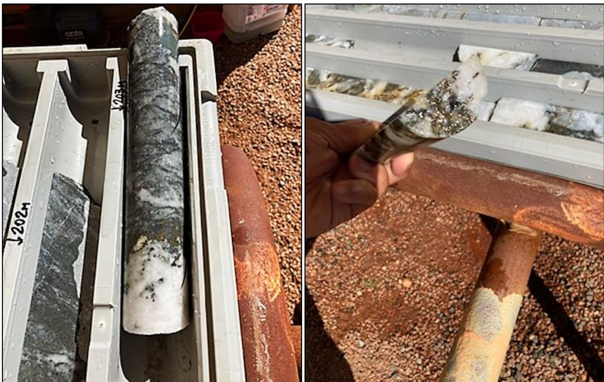
High-grade Bellevue Style quartz-sulphide mineralisation in hole KVRD025 grading 1m @ 13.45 g/t Au & 37.7 g/t Ag (202-203m shown).
