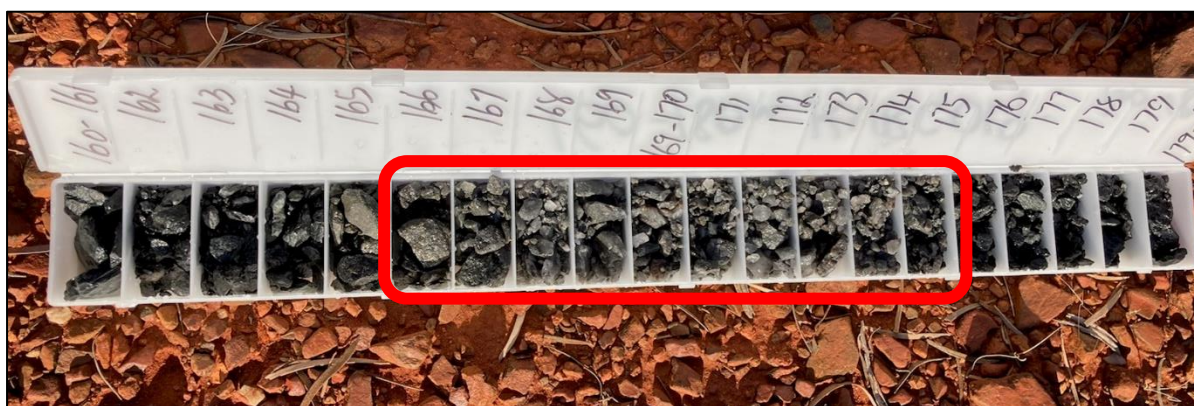
Figure 1: Drill hole KVRC019 with mineralised zone from 165-175m. Note abundant quartz veining, sulphide and bleached alteration in this zone.
