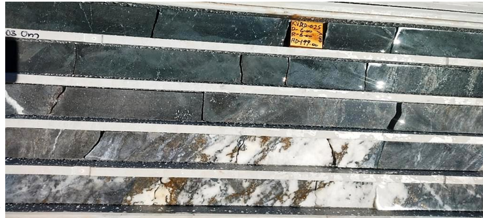
Drill core pictures top: Varying gold-silver bearing sulphide and quartz vein textures in the high-grade zone of KVRD026 which returned 6.6m @ 14.86 g/t Au & 21.79 g/t Ag, including 1m @ 27.60 g/t Au & 47.50 g/t Ag. These are the highest grades returned to date from the Coffey mineralised system.
