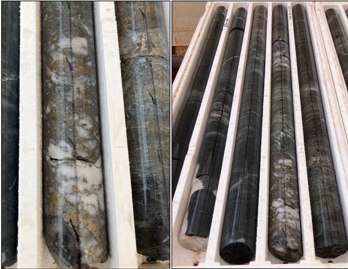
Bellevue Style mineralisation in hole KVDD033 with white quartz hosting sulphide mineralisation (212.0-216.7m shown).
