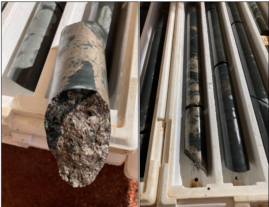
Semi-massive sulphides in the lower zone within hole KVDD034 (194.0m-204.8m shown).
