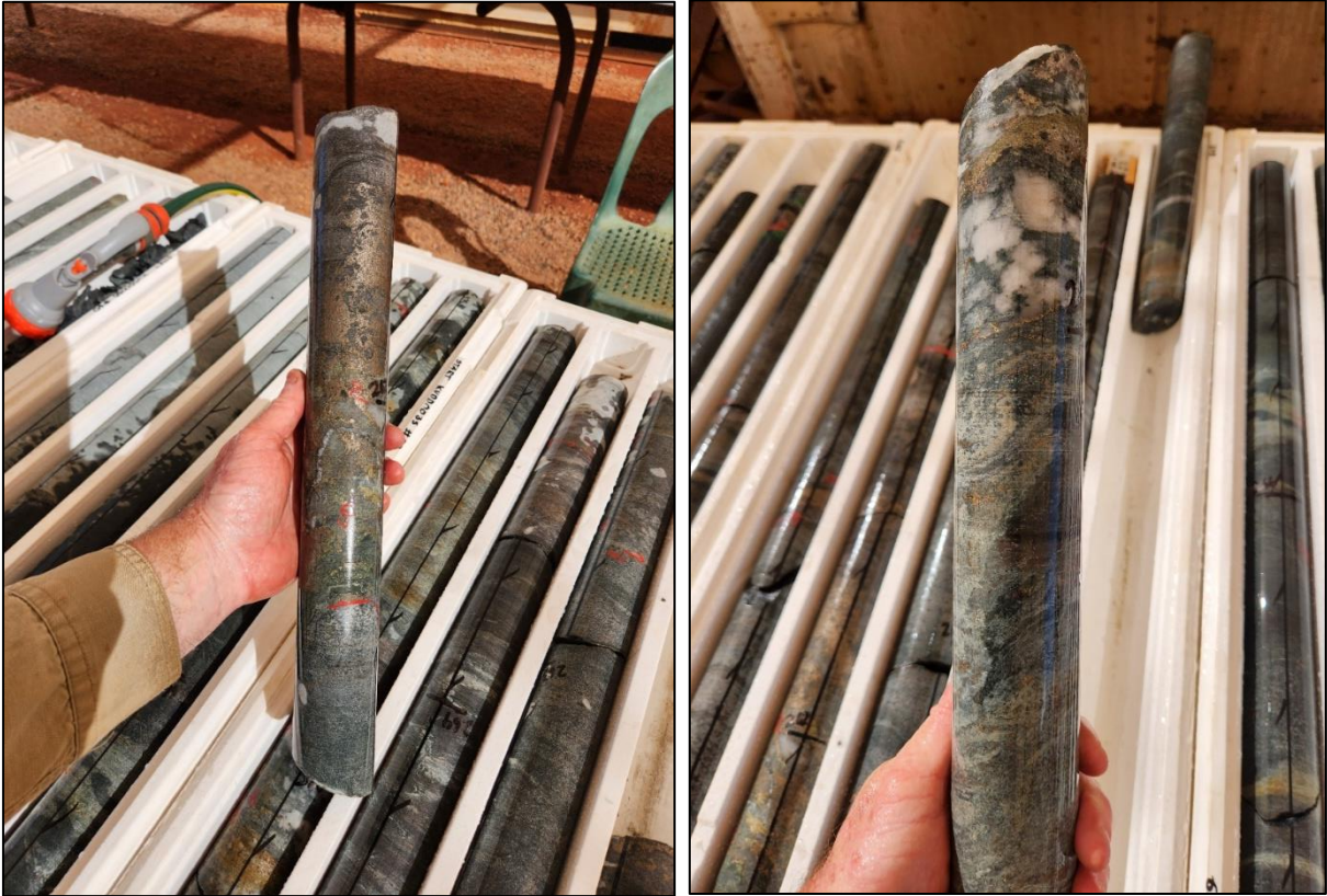
Figure 2 (left): Semi-massive sulphide and figure 3 (right) quartz breccia sulphides (right) within altered ore zone in diamond core hole KVDD0035.
