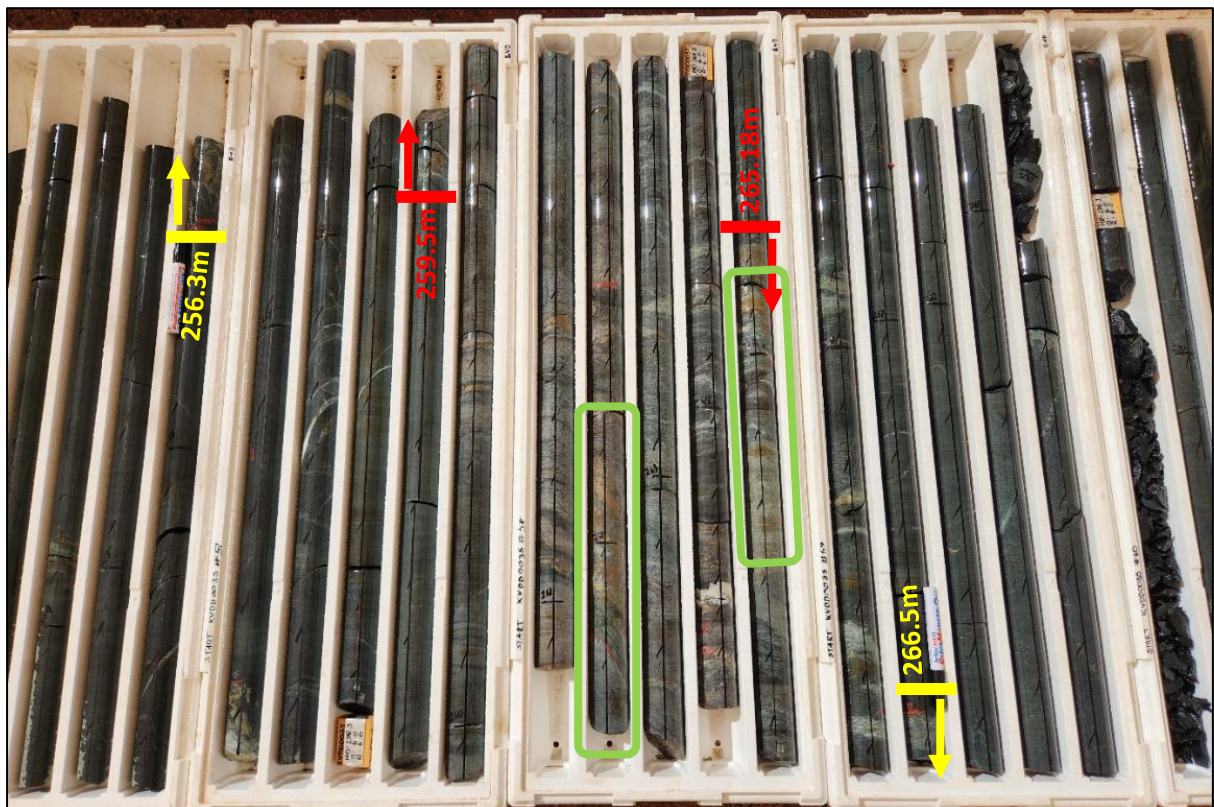
Figure 4: altered and mineralised zone within KVDD0035. Yellow marks and depths show the start and end of the main alteration zone with the red markers defining the heavily altered sulphide bearing zone
