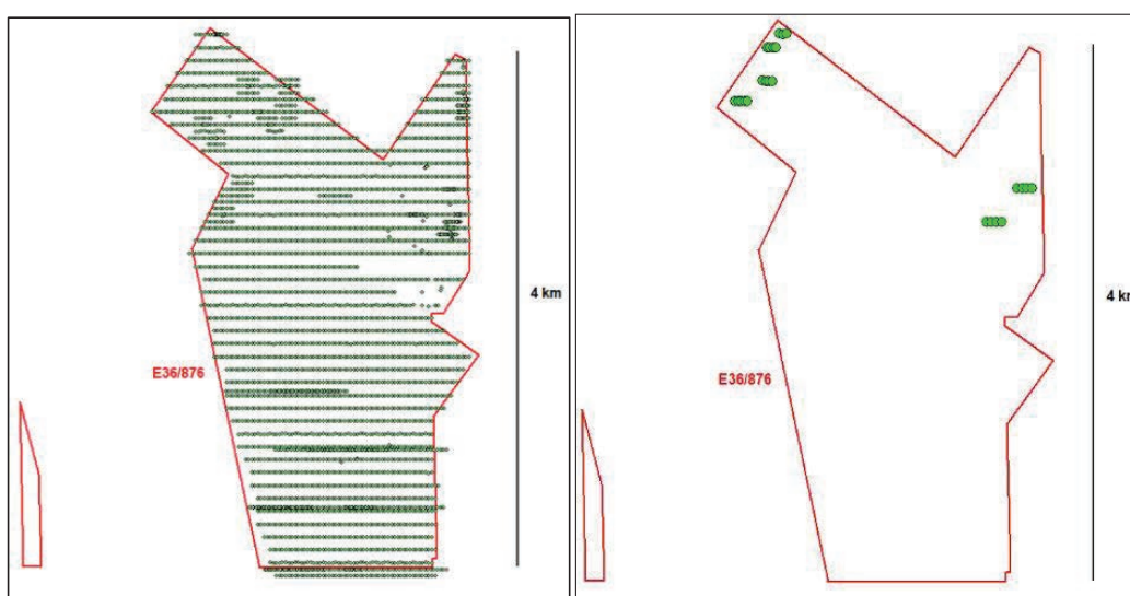
Figure 13: Barrick auger soil gold sample locations (left) and RCP drill collars (right), Kathleen Valley project area Source: Jones (2018)
